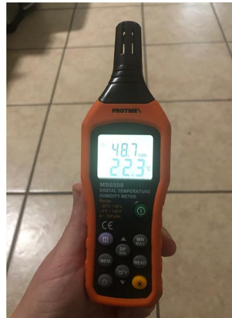
Figure 4: Use humidity detector to measure and control humidity. Image: BASTA
